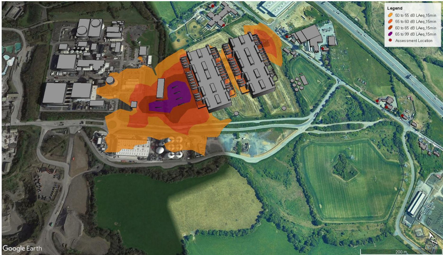
Figure 10.12 Scenario C – Proposed Data Storage Facility (current planning application) – Generator Testing Noise Contour (Extent of 50 dB(A))
