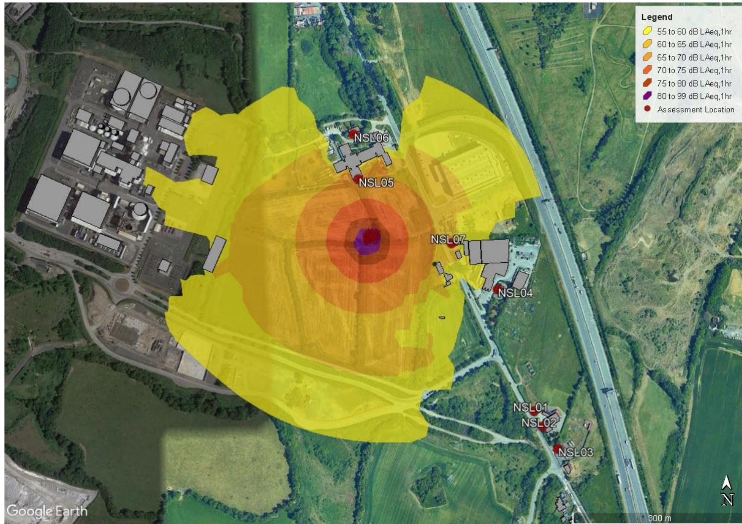
Figure 10.8 Construction Noise Contour – General Construction
